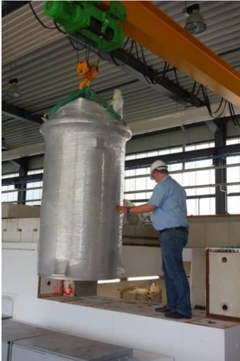
Small vertical test stand for testing up to 2-cell cavities or for use for the quadrupole resonator is delivered by Kriosystems
